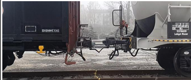
Coupler Validation up to 12 kp/h @ TÜV Süd, Görlitz 11/22 and 03/23
